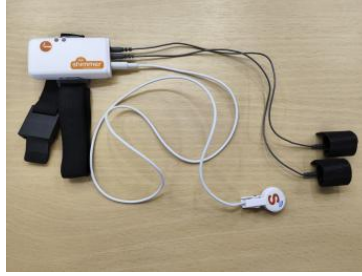
Fig. 3. Shimmer3 GSR+ Unit sensor.
