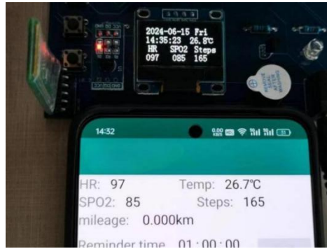
Fig. 9. Sensor data acquisition function test diagram
