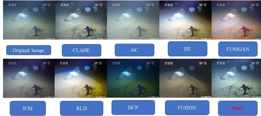
Fig. 1. Visualization of outputs from different underwater image enhancement algorithms. The Original Image is a randomly selected frame from the TrashICRA19[18] test video stream. Ours refers to the enhanced image using the FUNIE-CLAHE architecture. CLAHE[10], GC[19], HE[20], FUNIGAN[13], ICM[21], RLD[22], DCP[23], FUSION[24].
