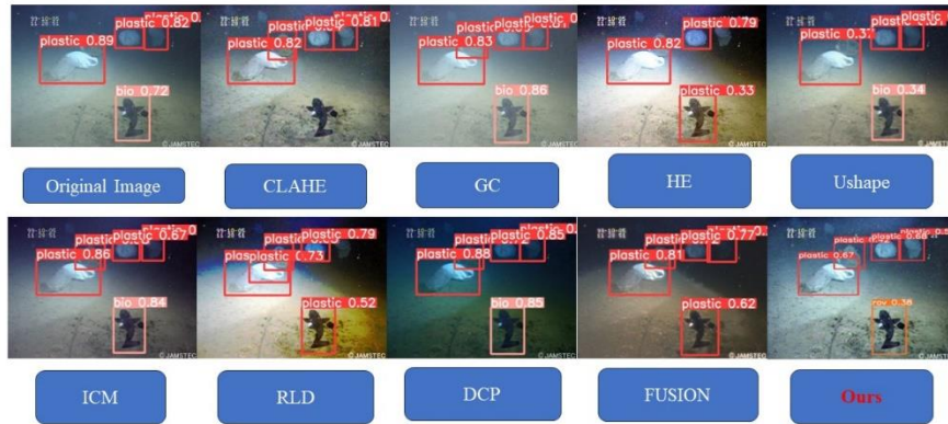
Fig. 4. Effect of Enhancement Algorithm on YOLOv5s Visualization. CLAHE[10], GC[19] HE[20], FUNIGAN[13], ICM[21], RLD[22], DCP[23], FUSION [24], Ushape [2].
