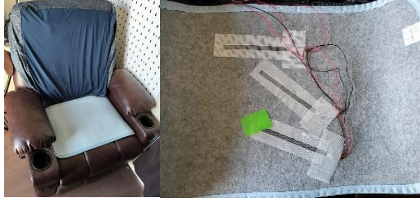
Fig. 4. (Left) Motorized recliner with sensors (Right) Cushion with pressure sensors
